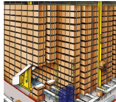
Captive Aisle System
